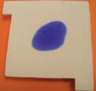
Back View: The blue ink seeped through the pores of the ceramic part
