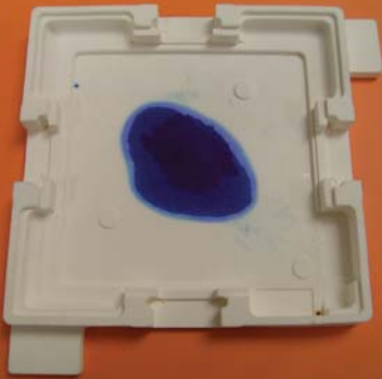
Front View: A few drops of blue ink were dripped on the porous ceramic injection molded part
